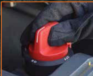
Battery cut-off switch
