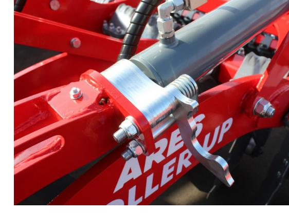
During transport, the roller is lifted on the machine by two hydraulic cylinders. When the machine is folded, the centre of gravity moves closer to the tractor and the threepoint linkage is relieved.
