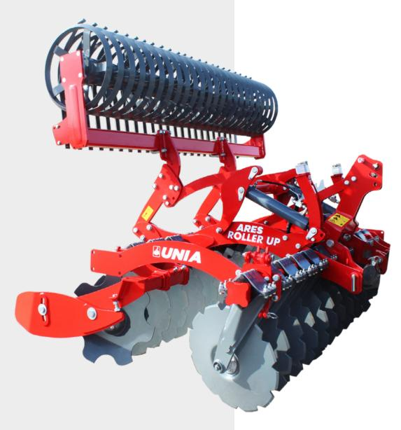
The working depth is set with patches placed on the roller lifting cylinders, 12 clips allow for precise adjustment. The maximum working depth is 18 centimetres
